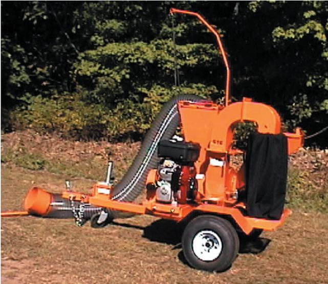
The Model 616CSV will process material in two different ways. Chip it **OR** Shred it! Then distribute in three different ways. Bag it, load it, **OR** recycle it! The chipper hopper has a 4" round wood capacity. Put leaves, prunings & trimmings up to 1/2" in shredder hopper. Choose chips **OR** shreds!
