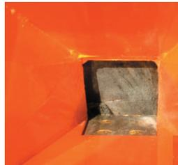
Chipper infeed opening at the disc is 4-1/8" x 6-5/16", and will easily accommodate up to 4" diameter round wood. Bed Knife is adjustable & sharpenable.
